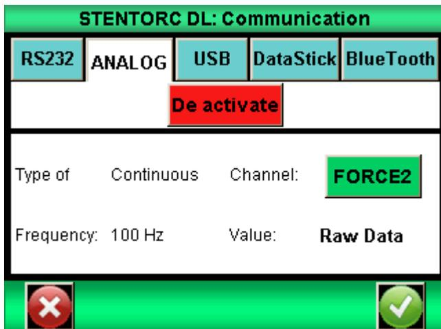
The Stentor II can send the analog data with a data rate around 100 Hz. The output is +/- 1V.
