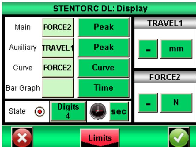
Configure the measuring screen in order to display the peak force on the main display area and the peak deflection value on the auxiliary display area :
