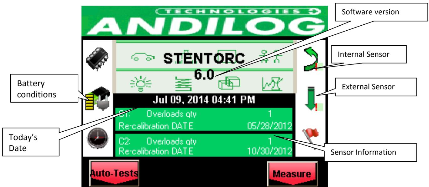
Battery condition: Display the battery condition
