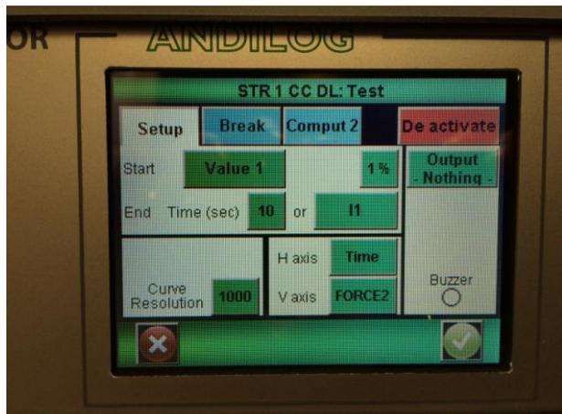
Configure the start condition on “VALUE1” with 1% detection
