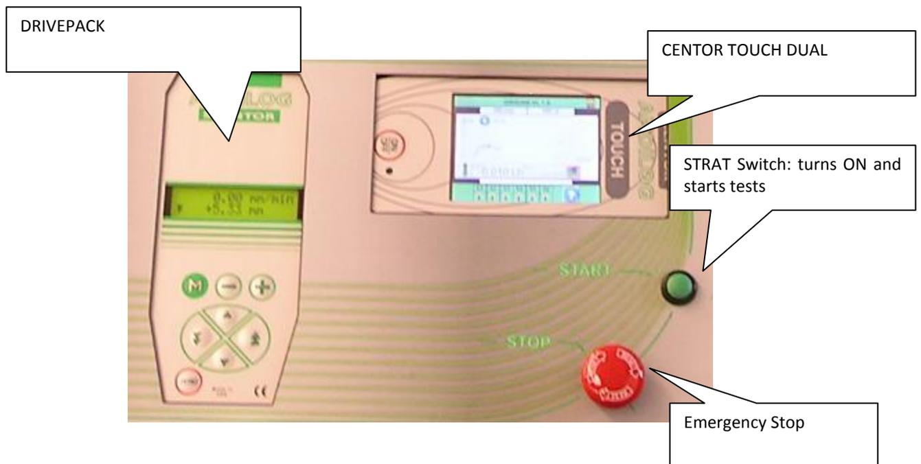
By switching ON the button on the side of the test stand and if the emergency button is not in down position, the DRIVEPACK will not turn ON. To start the CENTOR TOUCH, push its ON/OFF button: a general screen appears for 5seconds and then the main measure screen is displayed.
