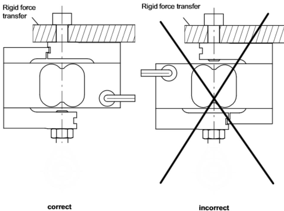
Load cell orientation during installation - load cell range from 2000N to 5000N:
