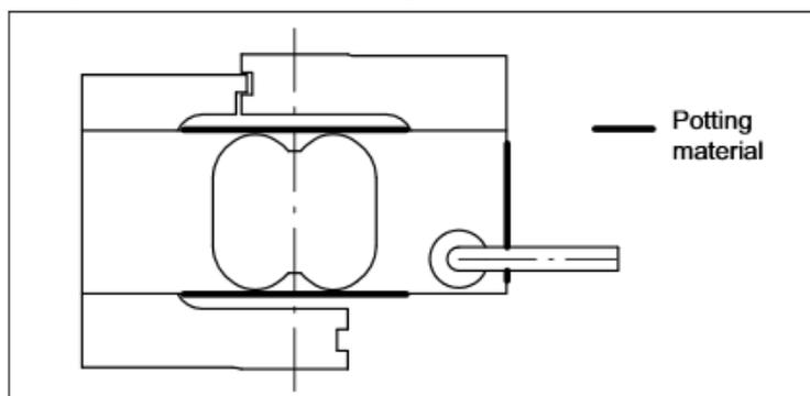
Strain gauge installation protection – load cell range from 2000N to 5000N:
