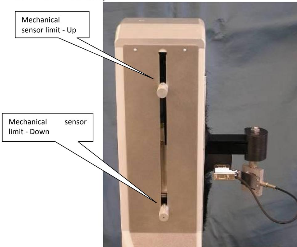
You can configure activation of your mechanical limits on the Drivepack menu at “Sensor stop
