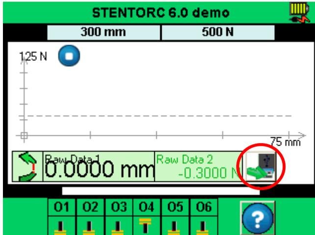
Once the DATASTICK communication is active, a USB icon appears on the main Measure screen:
