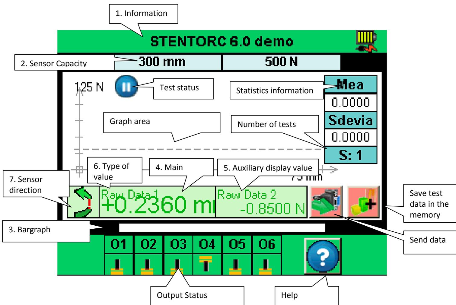
1 - Information: the version and type of the display is shown in this thin green bar as well as the battery indicator – note: Stentor do not operate on battery power... If you press his information bar, you will have access to the main menu.
