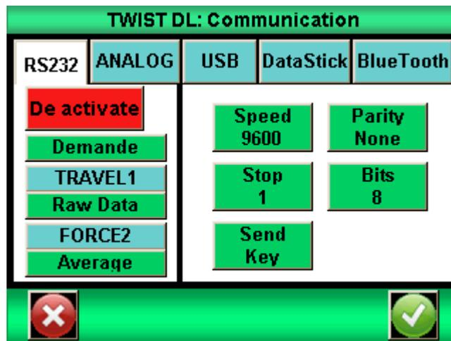
**Note:** Only one of the outputs can be used. All the other output will be deactivated. Be sure to select the tab corresponding to the output you want to use.
