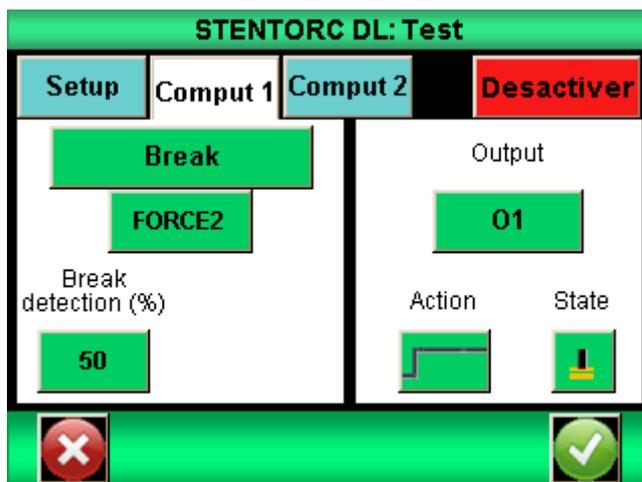
From the “Test” menu, “comput 1” tab, choose “break” from the available calculation and FORCE2. Set the percentage of the breaking force to 50% by example. Choose “Output” 01
