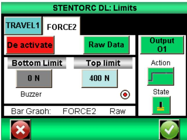
Touches the tab “FORCE2” from the limit screen. Set the upper limit to a 400N, enable the Output 1 and choose the
