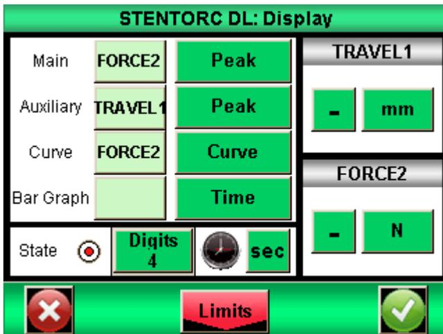
In this example, we are assuming we have a 500N load cell. We are displaying the peak force and maximum deflection values, and with a force limit protection of 400N.
