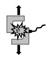
It is important that the measured values are generally below 90% of the sensor's capacity. Constant use of the load cell beyond 90% of its capacity can result in premature wear of the load cell. When the force gauge is used on a motorized frame, it is necessary to program the frame to stop when the force approaches the maximum capacity of the sensor. This limit must take into account the fact that at a
