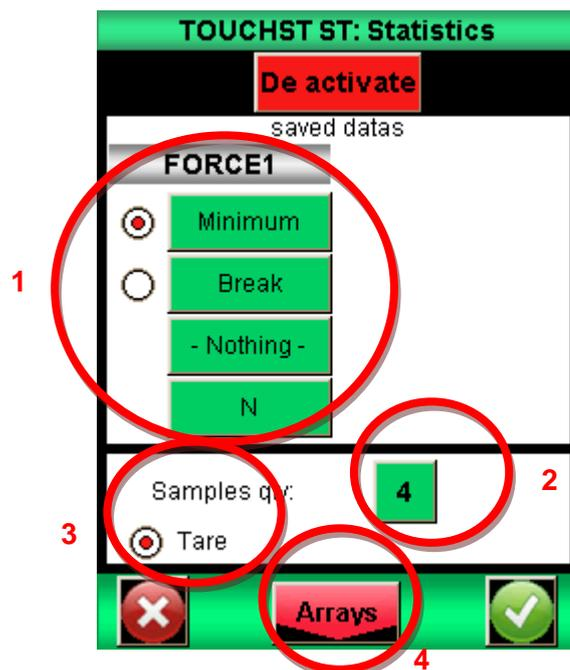
1: Select the desired result to be entered into the statistic arrays; you can choose 3 types of values to record: maximum, minimum, calculation1 or calculation2 for each channel. Select the units desired.
