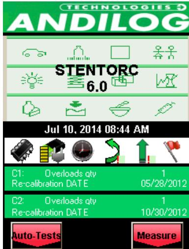
This screen is displayed after completion of internal tests and a minor or major defect has been found.
