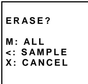
Press the left button (ZERO) to erase the selected sample or the complete set of measurements. If your sample includes several measures, they will be all deleted.
