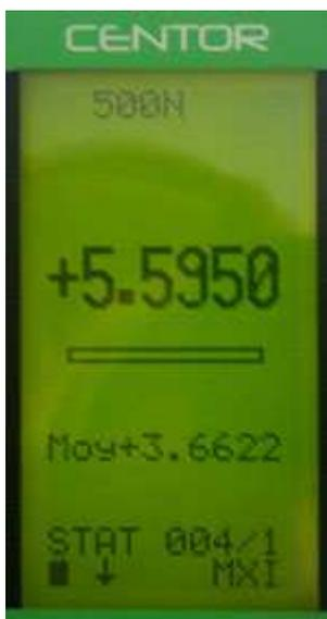
The measurement is performed by applying a force to the pressure sensor Centor. At any time the maximum is displayed in large characters on line 1. You can if you wish, display the current value instead of the maximum by pressing the top button (MAX).
