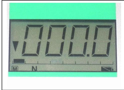
If a torque of more than 20% of the maximum capacity is applied via the plate, the display will show 'OVERLOAD'
