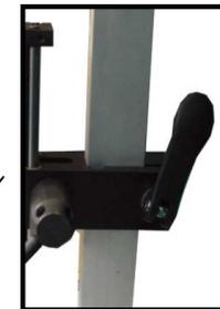
Adjust the position of the mounting plate to have your accessory align with the sensor rod
