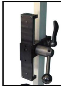
Adjust the height of the force gauge position thanks to the handle
