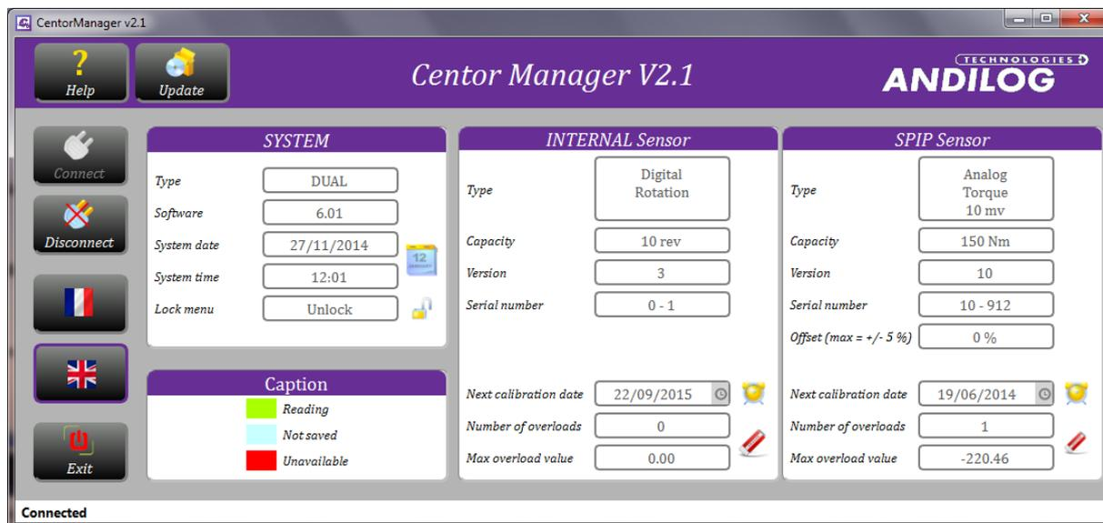
Centor Manager is very easy to use. Just plug your gauge and click 'Connect'. The software will automatically detect the communication port (RS232 or USB) and read the data of the gauge.
