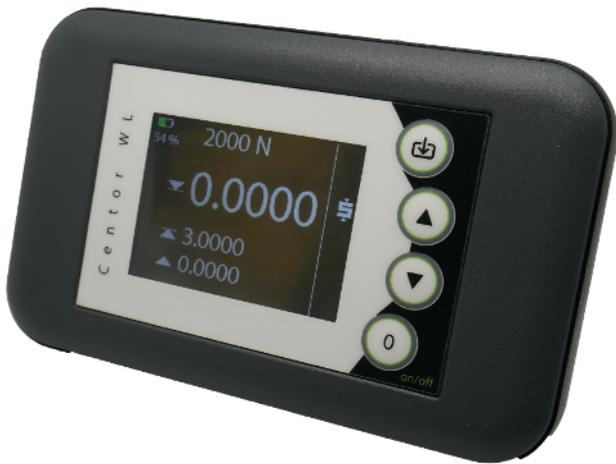
Thanks to Centor Wireless you can now use your force and torque sensors in Bluetooth. Compatible with the whole range of WLC sensors, the Centor Wireless is a simple wireless display for everyday measurement.
