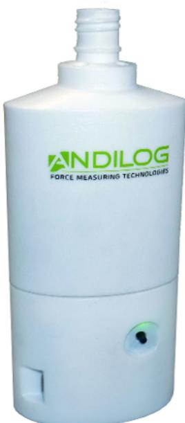
To control the quality of tightening of closures in production, most of the time, the loosening torque on the bottles is measured after the closure has been screwed or pushed in by the capping machine.
