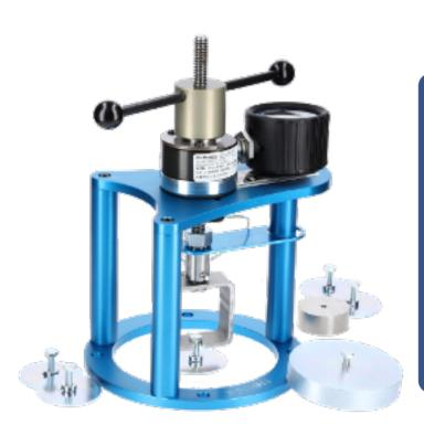
Com-Ten is an instigator in the validation of installation of insulation membrane, with the UPLIFT Tester, and the measurement of the bonding strength of coatings, with the ADHOR Tester. These products are designed to proof the good installation and adhesion properties in the field.
