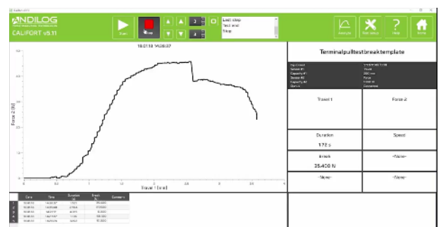
Example of a force measurement on the terminal until breakage
